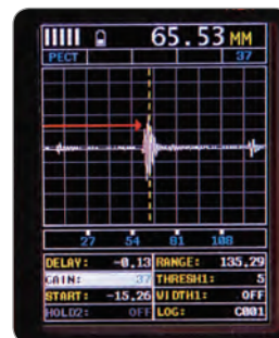
PECT Pulse - Echo Coating Mode Displays both the material thickness (PE) and the coating thickness (CT) at the same time.
