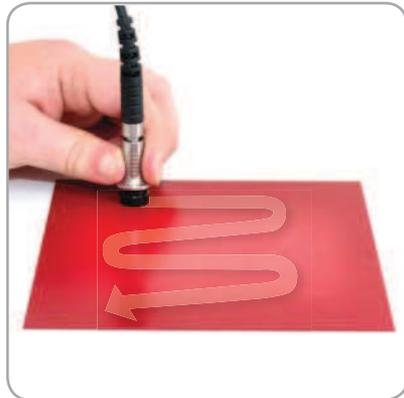
When the Scan Mode\* is selected users can slide the Ultra/Scan probe over the entire surface area. As the probe is lifted off the surface the gauge displays the average coating thickness value, the highest thickness and the lowest thickness values. Each set of three readings (average, high and low) can be displayed on the run graph and stored into the memory.
